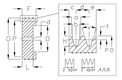
$\begin{array}{lll} D & = 108 \\ d & = 20 \\ F & = 82.0 \\ L & = 60 \\ Number of ribs = 4 \\ O & = 157.0 \\ P & = 150 \\ Type & = B \end{array}$
